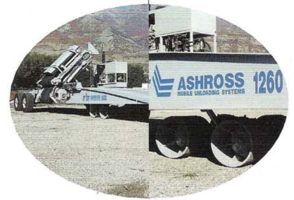
Drive-over deck sets only 32" off the ground at its highest point.
